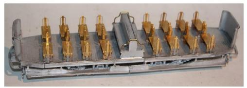
15. Fit the controller handles and one key to the controllers.
