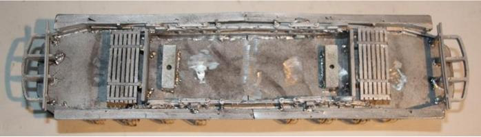
12. Very slowly and carefully bend the middle seat sides so that the lower section of the side slopes inwards in the same as the etched brass ones do, then fit to the seat.
