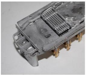
11. Fix the motor mounting blocks behind the ends of the lifetrays. Use the motorising unit to identify where they need to be fixed.
